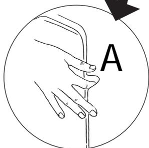
1. Lift both catches on either side of the door at the same time. Fig 1.
